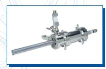
mechanical valve to limit the conductance from the evaporation (sublimation) reservoir to the growth chamber. A constant temperature may be maintained and the valve position is used to control the flux, allowing for a stable and reproducible deposition rate.
