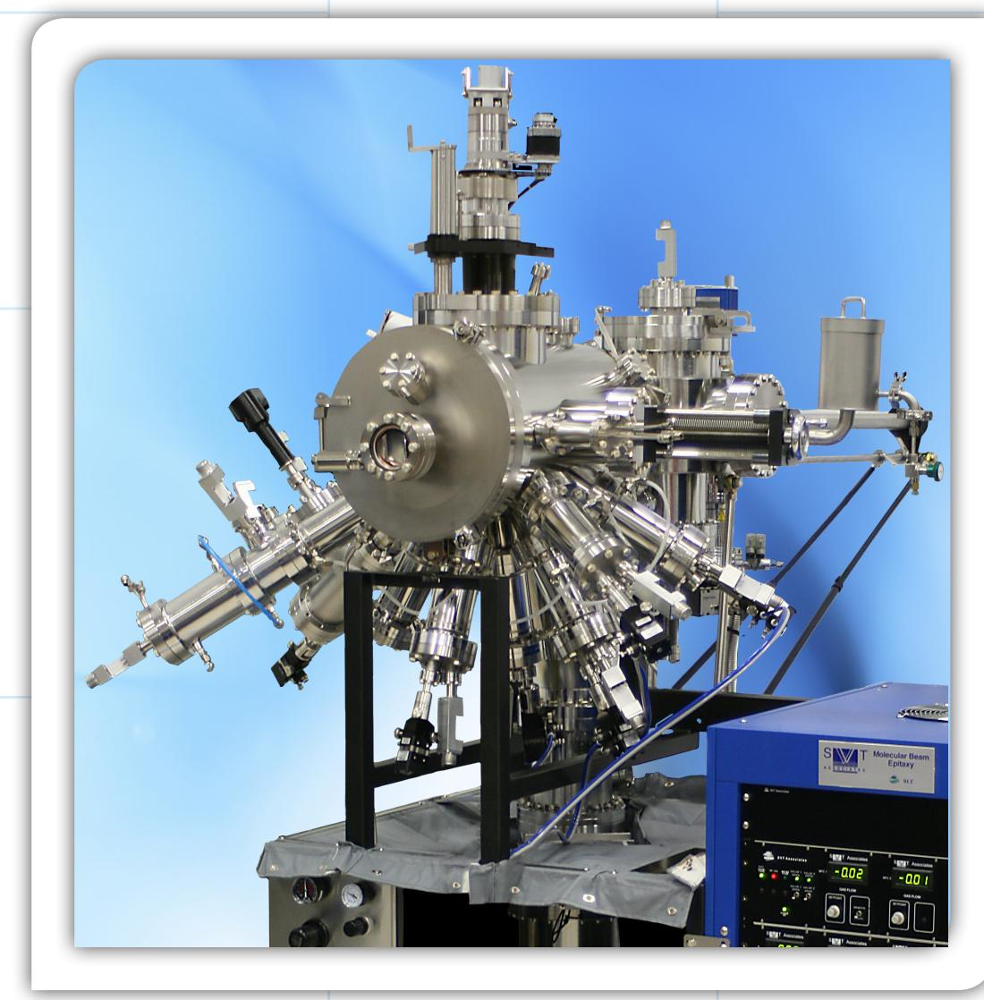
The SMART NanoFab MBE system is the perfect combination of small footprint and large capability. The table-top UHV chamber includes a series of ports to accommodate a wide selection of deposition sources and process monitoring tools.
