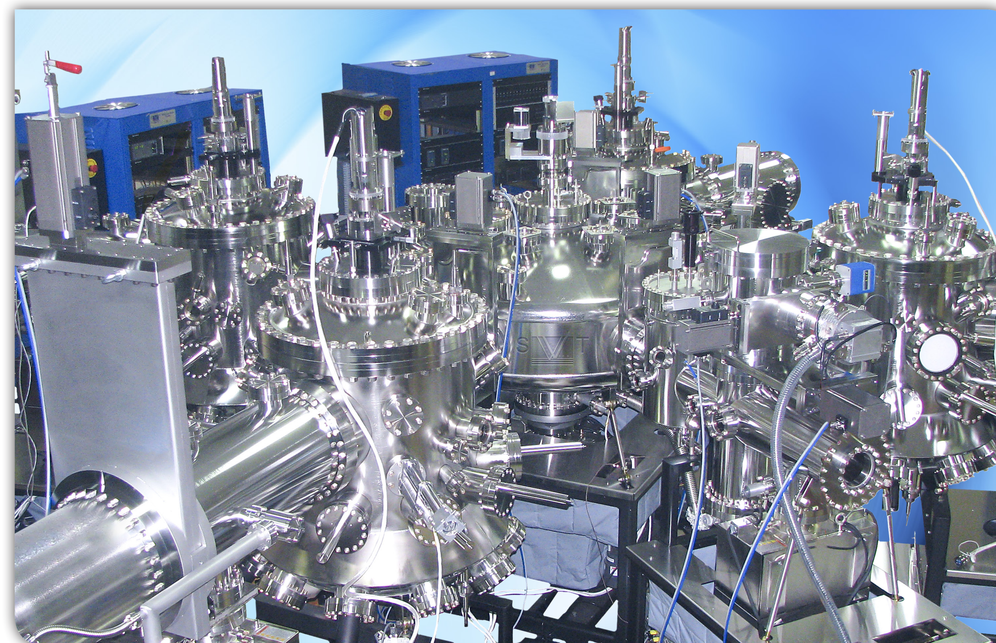
MBE Modules with UHV Cluster Tool
