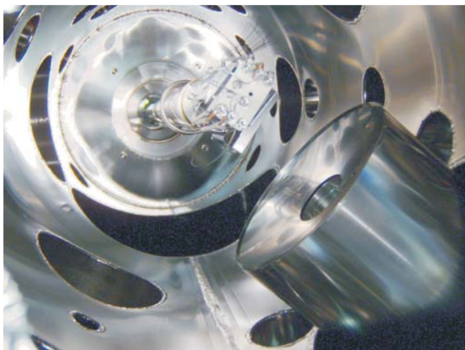
UHV Target and Sample Shown within MBE Growth Chamber
