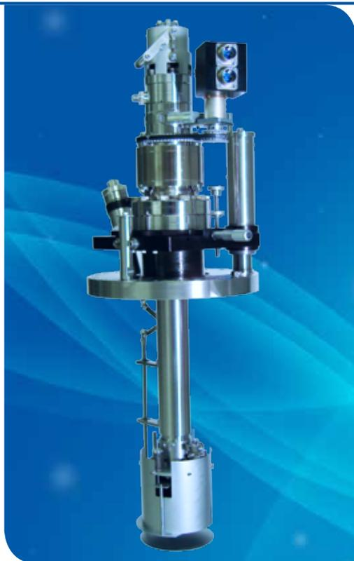
Standard 3" Stage, Filament, and Integrated Shutter
