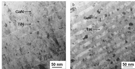
Cross-sectional TEM images of (a) a TiN (5 nm)/GaN(30 nm) multilayer grown on a (0001) sapphire substrate and (b) a TiN (20 nm)/GaN (variable thickness) multilayer grown on a (100) MgO substrate.
