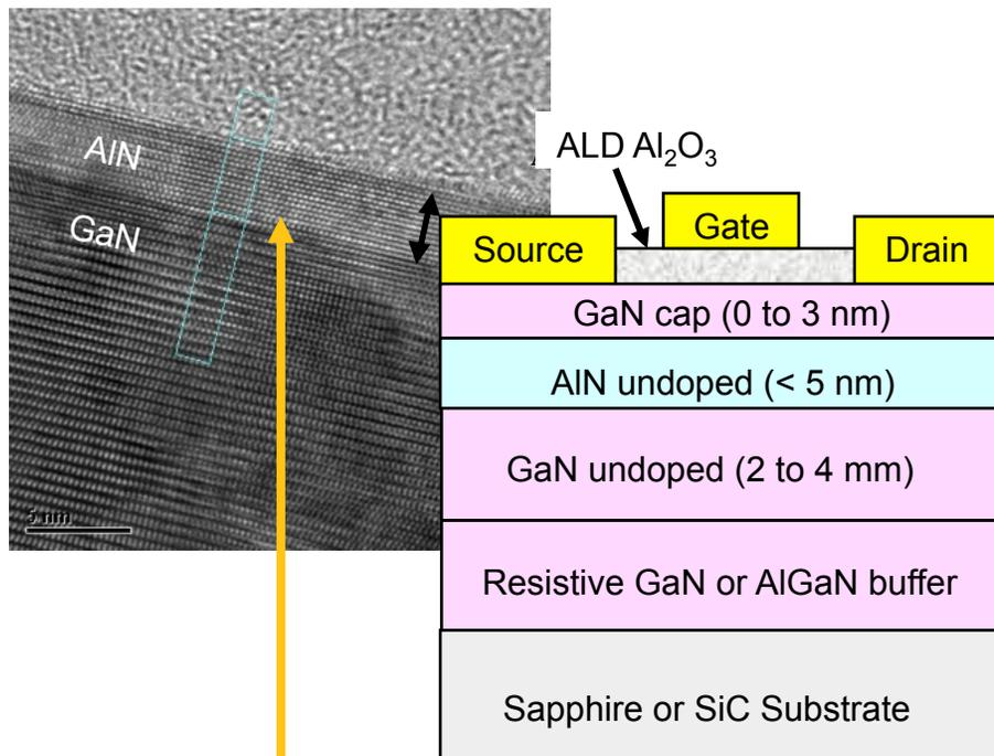
Nanometer scale AlN barrier layer requires low-damage gate-oxide deposition by ALD
