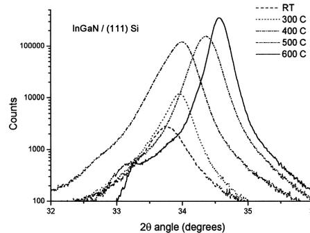
XRD  $\theta$ - $2\theta$  scan for  $\text{In}_x\text{Ga}_{1-x}\text{N}$  films grown on (111) Si at different temperatures
