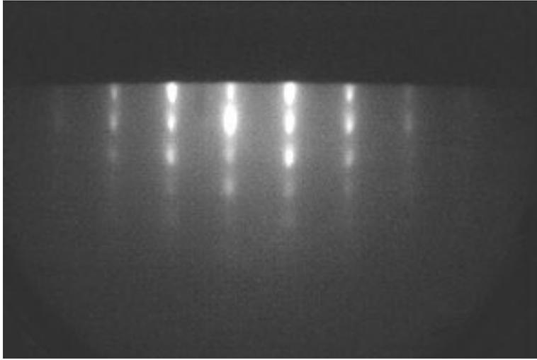
RHEED pattern from the 130 nm thick AlN film with the electron beam incidence along AlN[11-20] direction
