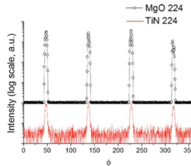
X-ray phi scans about MgO 224 and TiN 224 reflections of a 2.35 μm thick TiN(1.4 nm)/GaN(1 nm) multilayer grown on MgO.
