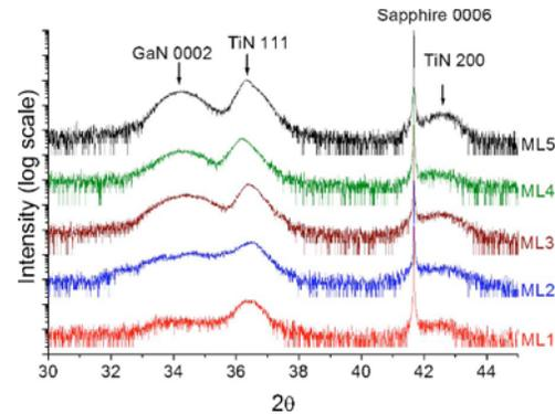
w-2θ symmetric θ-2θ x-ray scans obtained from the TiN-GaN multilayers grown on sapphire with periods of (a) ML1, λ=3.4 nm, (b) ML2, λ=6.8 nm, (c) ML3, λ=15.9 nm, (d) ML4, λ=19.1 nm, and (e) ML5, λ=22.5 nm.
