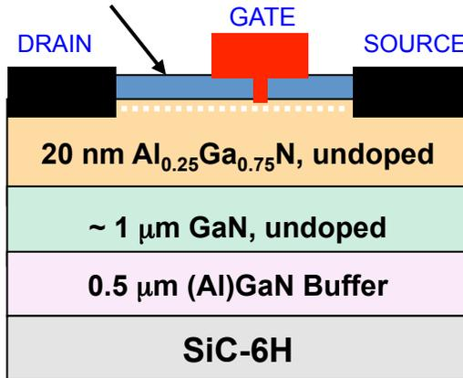
$L_G = 0.25 \mu\text{m}$  or  $0.12 \mu\text{m}$
