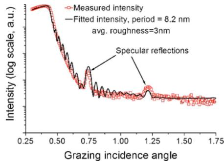
X-ray reflectivity spectra and the fitted data for sample ML2.
