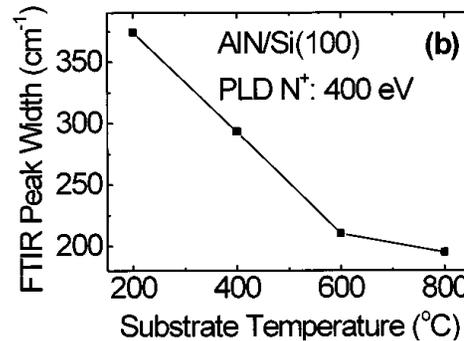
FTIR spectra of AlN thin films deposited under different substrate temperatures: 200, 400, 600, and 800 °C.
