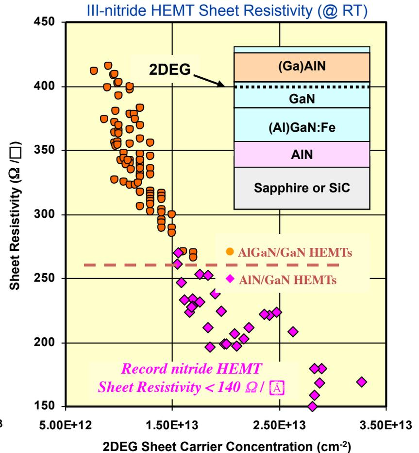
The channel conductivity of high-quality AlGaIn/GaN HEMTs is limited to above  $\sim 250 \Omega/\square$  by both surface roughness and alloy scattering. We have been able to overcome this barrier by growing high quality AlN/GaN HEMTs on sapphire and SiC with record properties as shown in above figures.
