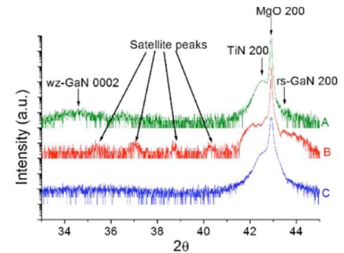
w-2θ & x-ray scans obtained from three different period TiN-GaN multilayers grown on MgO(100) substrate. The multilayer or superlattice period is given as A=18.4 nm (with TiN=12.2 nm/GaN =6.2 nm), B=5.5 nm (with TiN=4.3 nm/GaN=1.2 nm), and C=2.4 nm (with TiN=1.4 nm/GaN=1.0 nm)
