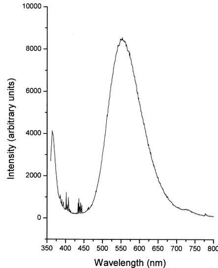
PL spectrum at room temperature for GaN/sapphire sample grown at 600 °C.
