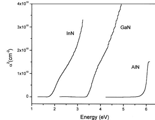
Square of the absorption coefficient as a function of photon energy, calculated for InN, GaN, and AlN thin films. Linearity indicates a direct transition bandgap. Onset of linearity is at bandgap energy value.
