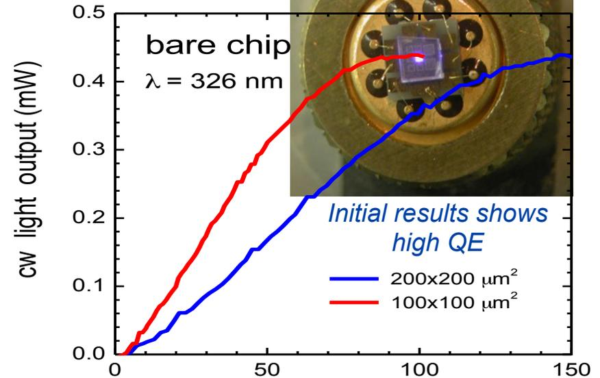
Compositional inhomogeneity in InGaN-based LEDs is known to enhance blue/green emission by increasing carrier localization. High growth temperatures required for AlGaN-based UV LEDs make In incorporation difficult. Recent work at Army Research Lab have shown dramatic improvement in UV-LED efficiency by creating Nano-compositional inhomogeneities in AlGaN active layer.
