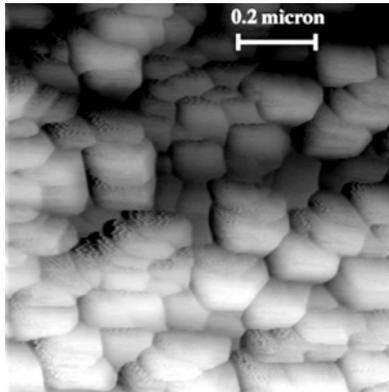
AFM image of an AlN/sapphire sample grown at 700 °C. The imaged square has a 1mm side
