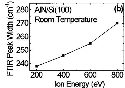
FTIR spectra of AlN thin films deposited under different nitrogen ion beam bombardment: 200, 400, 600, and 800 eV. The substrate was at room temperature
