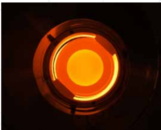
2" Sample Heater for Oxide MBE. The Oversized Filament Ensures Uniform Heating even to the Edges of the Substrate up to 1,000 °C
